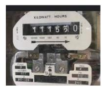
The meter can be read from left to right, including all leading zeros. If a dial appears to be between numbers, record the lower number - except when the dial sits between 9 and 0, note down 9. If your meter has two readings marked with an L and H, please read both, left to right. If you have this meter type, submit both numbers.
