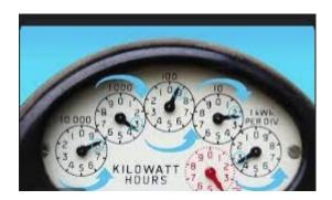
Read each dial from left to right. Please note that the dials alternate in direction. When a dial is between two numbers, you should write down the lower number. If its between 0 and 1, write down 0, but if it points between 9 and 0, write down 9. If the pointer is resting directly on a number, look at the dial to the right. If this number hasn't passed 0, then the original dial hasn't passed the number yet and you should note the lower number.
